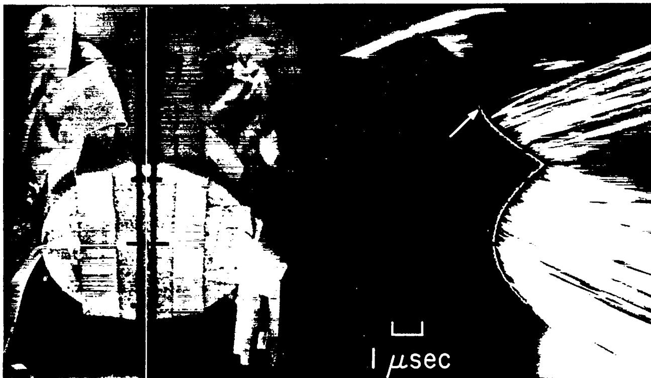
Fig. 9. Left: Still photograph of Amatex cylinder as viewed by rotating-mirror camera. The camera slit position is shown by the white vertical line. The booster pellet was located on the upper plane surface of the cylinder. Right: Detonation record. Time increases to the right. The white arrow indicates breakout of detonation at the cylinder wall.
